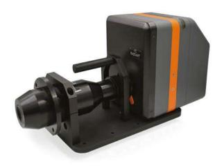
View angle measurements are critical to automotive displays, which must be flawless when viewed at an angle. Radiant's FPD (flat panel display) conoscope lens provides angular resolution of 0.05 degrees per CCD pixel for high-precision measurement of luminance, radiance, angular contrast, CIE chromaticity coordinates and correlated colour temperature (CCT) at all viewing angles up to ±70 degrees.
