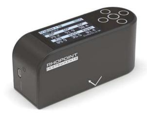
While standard glossmeters only measure how much light is reflected from a surface, the IQ-S profiles how light is reflected from a surface and characterises effects which dramatically reduce appearance quality, such as reflection haze.
